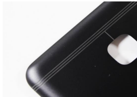
Exhibit 4: Micro Slot Antenna
